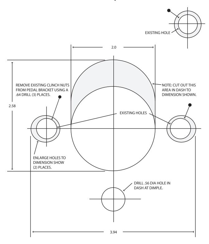
This template is used to modify the fire wall when converting from manual brakes to factory type power brake booster on 67-70 Mustangs and Cougars. Most important thing is the big hole for the booster must be raised up from the original master cylinder hole position.
