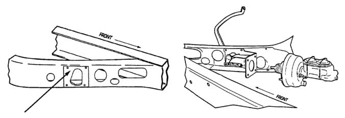
Line up holes in the paper template with the holes in the frame. Top of template should be parallel with top of x-member. Mark and cut out excess metal that is not covered by template. Please refer to Power Brake Booster and Master cylinder instructions for the remainder of the kit.
